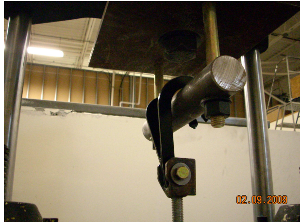
Photo 2 –Test set-up on 2”round bar
